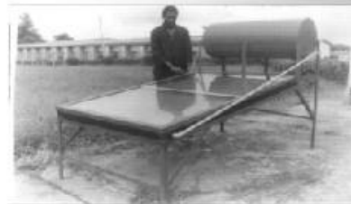
Solar Water Heater developed by NCERD
