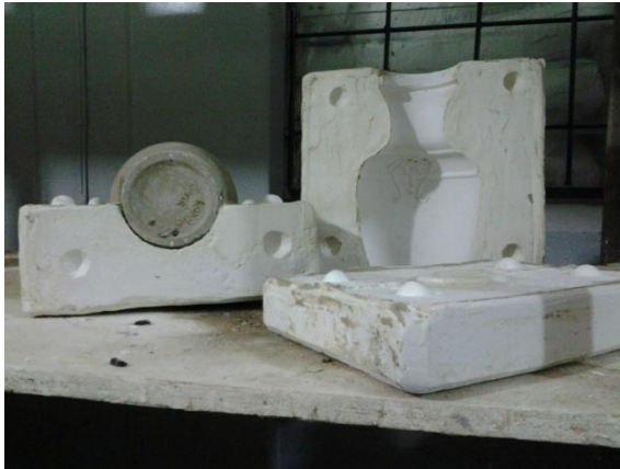
An example of three - piece mould
